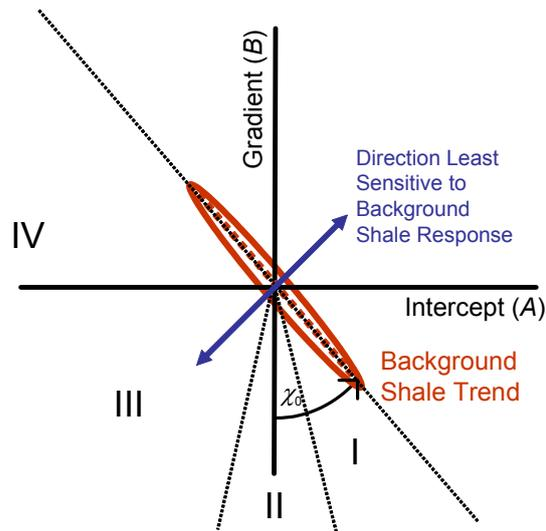
Figure 1: Schematic AVO crossplot showing regions corresponding to Class I-IV reflections. The background shale trend plots at an angle of  $\chi_0$  from the negative  $B$  axis.
